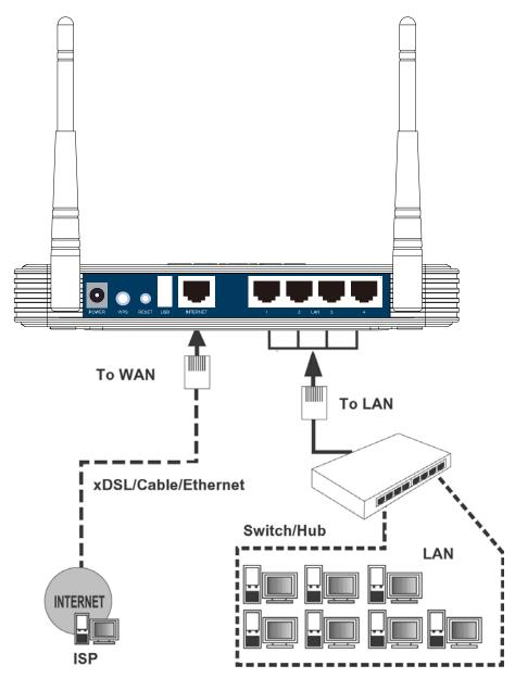
Figure 2-1 Hardware Installation of the TL-WR1042ND 300Mbps Wireless N Gigabit Router
